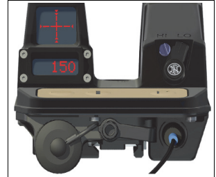
Fig. 3.s - Reticle moving and range appearing
