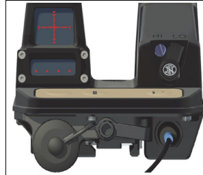
Fig. 3.r - Activating the aiming reticle
